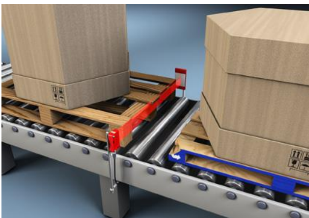
Figure 3 a/b. Reliable detection of pallets of varying sizes (left) and of objects with curved contours.
