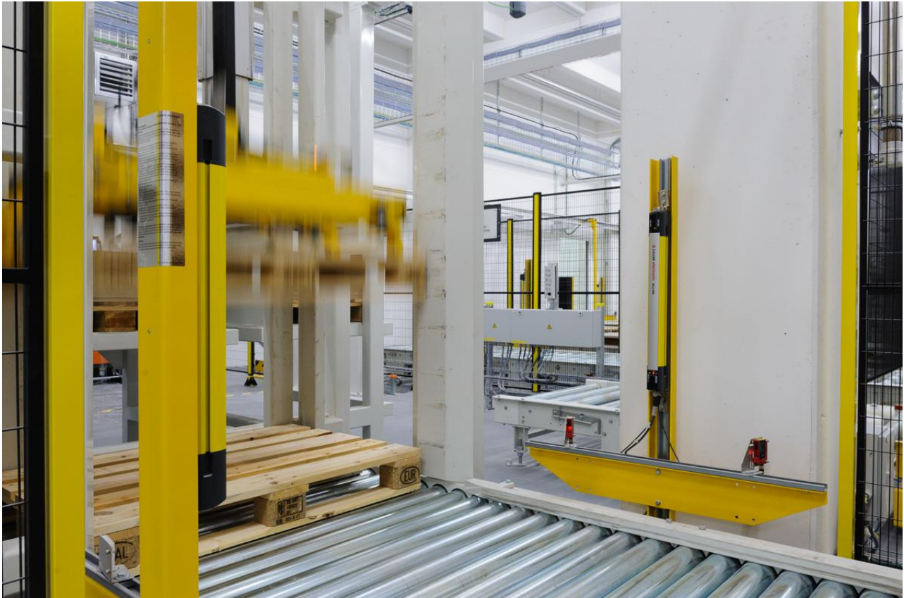
Figure 4. The light-band also makes the RK 46C VarOS ideal as a muting sensor.
