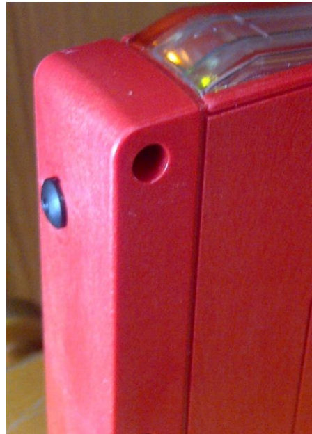
Figure 2. easyhandling: the sensitivity is set via the black teach button on the sensor housing – the sensor state remains highly visible.
