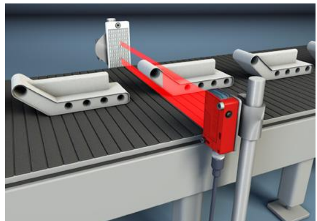
Figure 3 a/b. Reliable detection of pallets of varying sizes (left) and of objects with curved contours.
